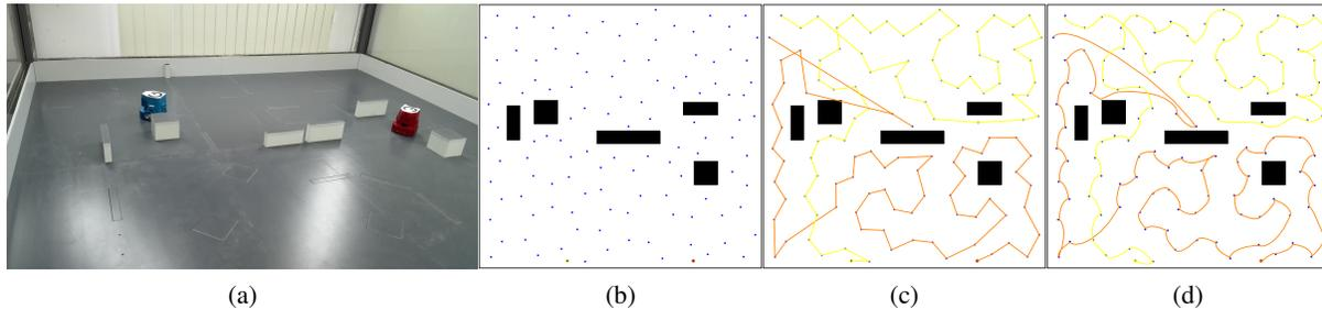
Fig. 4: Real experiment. (a) The robots performing the mission. (b) The map with generated goals (note that obstacles were inflated by Minkowski sum enabling to plan non-colliding paths for circular-shaped robots). The starting positions are highlighted in yellow and orange. (c) Planned routes. (d) Trajectories traversed by robots.
