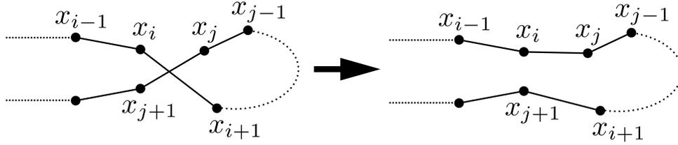
Fig. 1: 2-opt operation: edges  $(x_i, x_{i+1})$  and  $(x_j, x_{j+1})$  are removed and replaced by edges  $(x_i, x_j)$  and  $(x_{i+1}, x_{j+1})$ .
