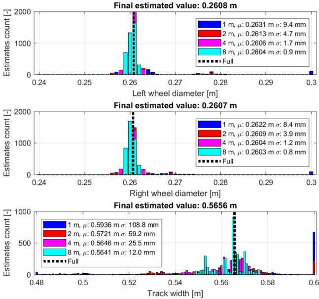
Fig. 8. Histograms of estimated chassis parameters depending on the sub-trajectory length
