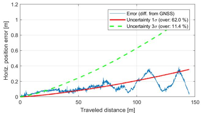
Fig. 11. Horizontal position error of the odometry on the validation trajectory
