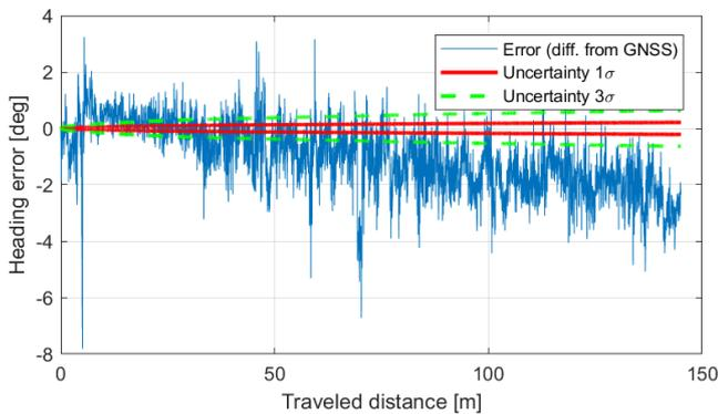
Fig. 12. Heading error of the odometry on the validation trajectory
