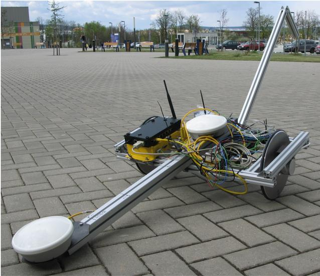
Fig. 2. Platform with the installed instrumentation needed for the calibration of the chassis
