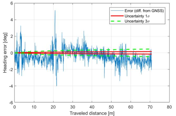
Fig. 6. Heading error of the odometry on the estimation trajectory
