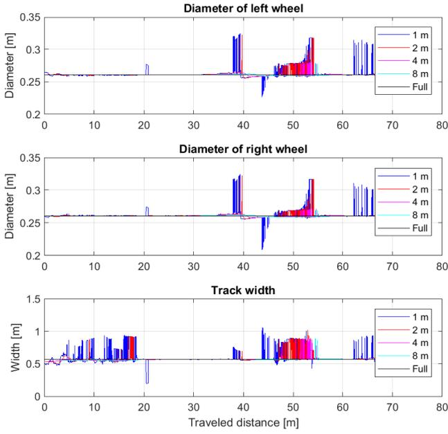
Fig. 7. Estimated chassis parameters along the trajectory according to the sub-trajectory length
