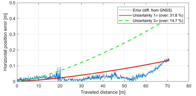
Fig. 5. Horizontal position error of the odometry along the estimation trajectory from Fig. 4
