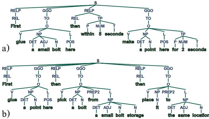
Fig. 8. (a) A task template “glue a small bolt” described by a sentence “First glue a point here then pick a bolt from a small bolt storage then place it to the same location”. (b) Resulting tree (abstract representation of sentence) gained from parsing the sentence “First glue a small bolt here then within 5 seconds make a point here for 2 seconds.” The task template “glue a small bolt” is reused in this sentence.
