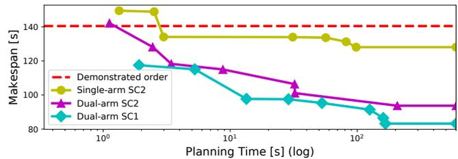
Fig. 6. Makespan vs. solving time for showcase 2 (gluing action in given locations with constraints on the the ordering) compared to the showcase 1 (dropping the ordering constraints), single-arm execution, and single-arm execution in the demonstrated order.
