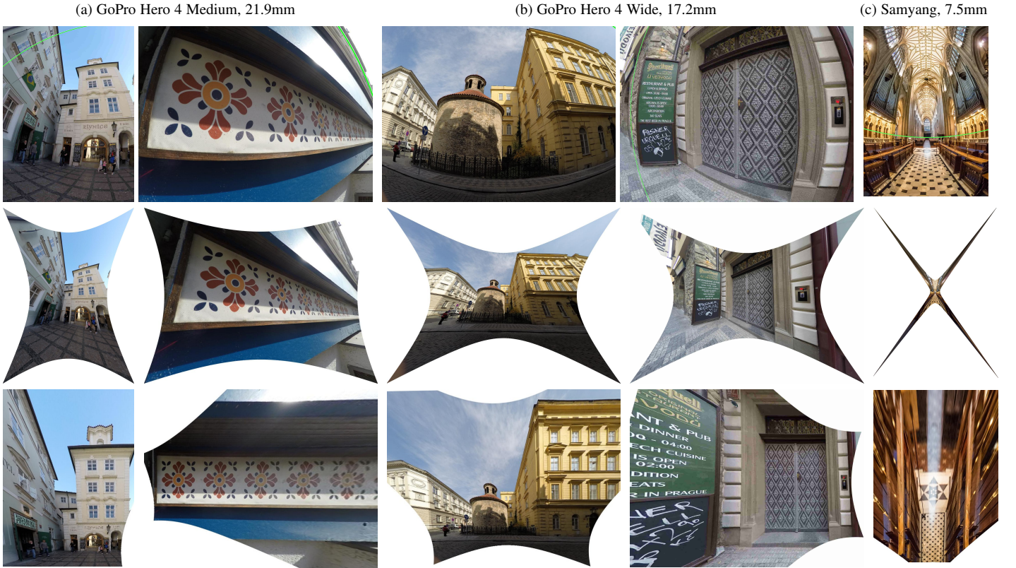
Fig. 4. The proposed solvers give accurate undistortions and rectifications across all fields-of-view. The distorted image of the vanishing line is rendered in green. Left-to-right with increasing levels of distortion: (a) GoPro Hero 4 at the medium-FOV setting, (b) GoPro Hero 4 at the wide-FOV setting, (c) and a Samyang 7.5mm fisheye lens. The outputs are the undistorted (middle row) and rectified images (bottom row). Note the stability of the undistortion estimates for the GoPro images. The rotunda image is rectified from features extracted mostly from the wrought iron fence below the rotunda. Focal lengths are 35mm equivalents.
