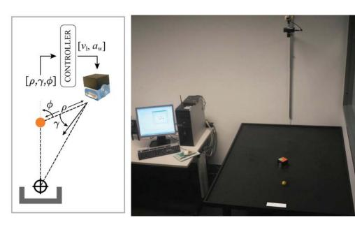
Figure 5: Definition of variables for the Ball-Pushing problem (left), and, a picture of the experimental setup implemented for testing the Ball-Pushing behavior (right).
