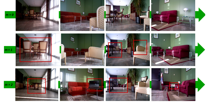
Fig. 4. Sample of images captured by the robot in three different mapping sessions. Changes as movement of chairs, presence of new objects such as cups or bottles are introduced between mapping sessions (red boxes).
