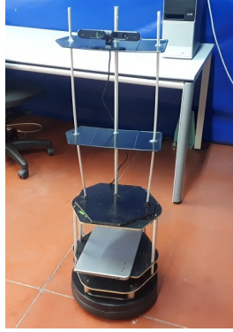
Fig. 4. Mobile robot TurtleBot 2 equipped with a camera used in the experiments.
